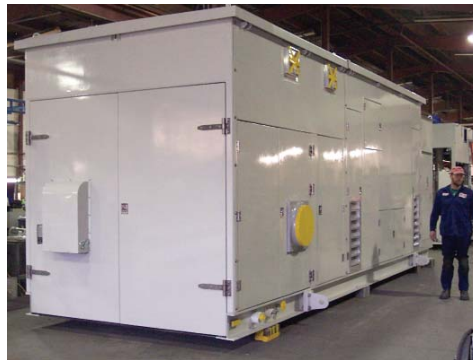
Fuel Cell Power Plant
