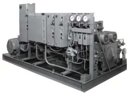
Water Injection Skid
